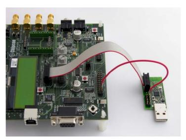
Figure 2 CC2511 Dongle powered from SmartRF04EB
